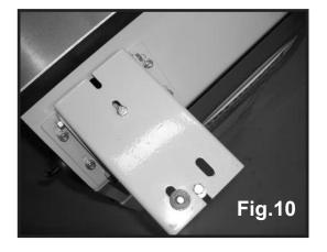
Loosen the four M6 bolts using a 10mm spanner (fig10) then slide aluminium extrusion into place (fig 11 and 12) then re-tighten the M6 bolts.
