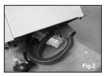
With assistance tilt the machine and remove all accessories from inside the machine (fig 2). Remove the two metal plates from the base of the machine using an 8mm hex key (fig 3)
